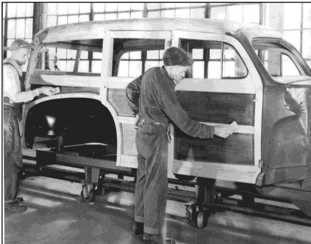
Block sanding the body between coats of varnish.
