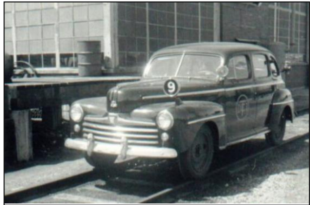
A 1947 Ford track inspection car - at this time, the DT&I was owned by the Pennsylvania RR, but maintained close ties with Ford Motor Company and the rest of the auto industry
