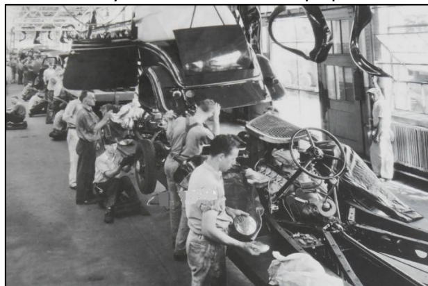
In this 1934 assembly line photo the body of this Roadster (?) is about to be lowered onto the chassis. The front fenders are already attached.
