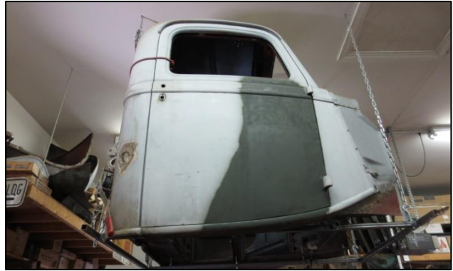
Dave welded up a special fixture to hold the cab while suspended.
