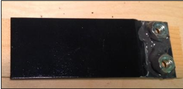
The flipper with the nuts attached using JB-Weld.
