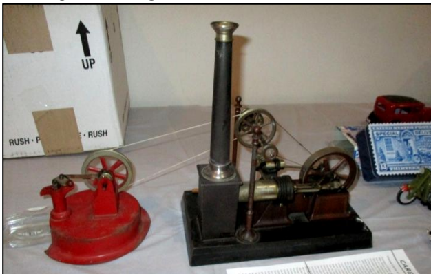
The steam engine powered the red pump on the left.
