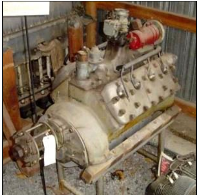
A barn find that beats all others! Instead of a transmission there's a 2:1 reduction for the propeller.
