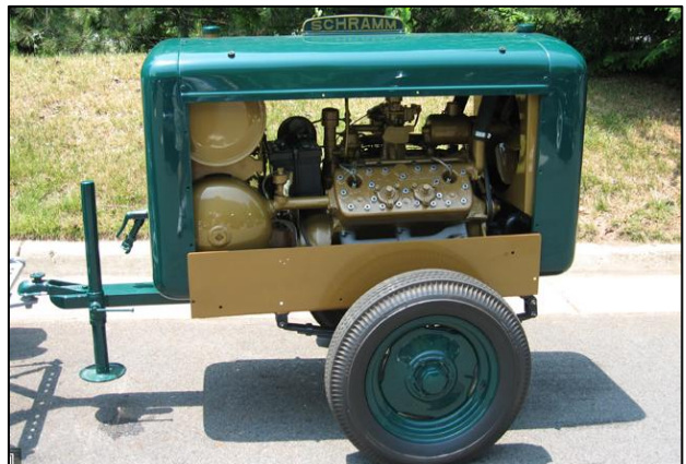
The front and rear cylinder run the engine while the center two compress air – just the opposite on the other side.
