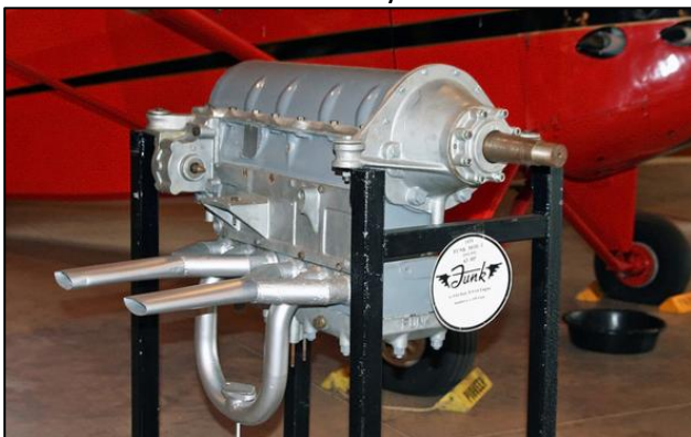
The Funk Brothers designated their highly modified Ford Model B engine as their Model E.
