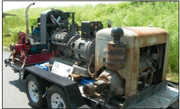
This trailer has three KR Wilson power devices on it. The front and back units are power take-off units which might be used to power a saw mill or something similar. The center unit is a flathead powered generator.
