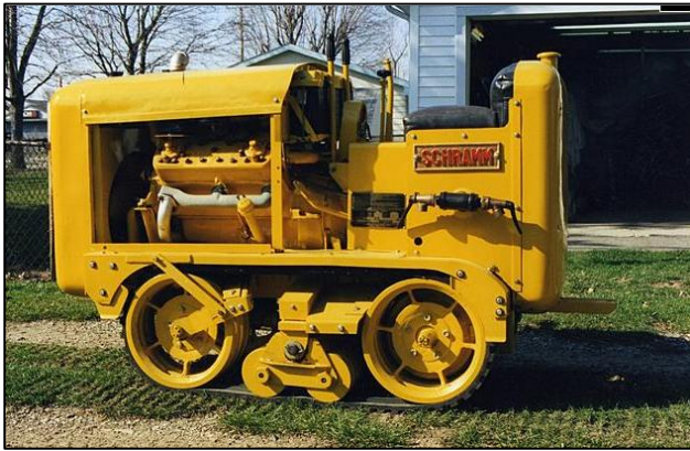
1948 Schramm model 60 crawler (Fordair 60). It runs on 4, compresses on 4. It's 1 of 150 made by Schramm.
