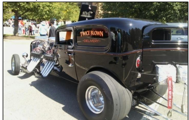
This is what I mean by "just about anything:" twin blown Keith Black hemis power this rodded '32 Panel Delivery.
