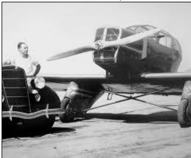
That black thing between the landing gear struts is the radiator.
