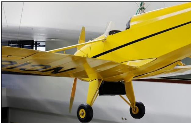
That black thing between the landing gear struts is the radiator.
