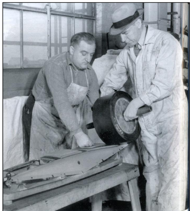
Craftsmen applying the grain to a 1939 Ford dash in this Ford Archives photo. Check out the guy on the right who has the top shirt buttoned and wearing a tie and a fedora.
