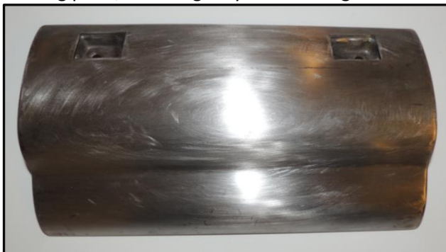
A 1946-8 glove box door has been stripped, sanded and cleaned with good prep solvent.
