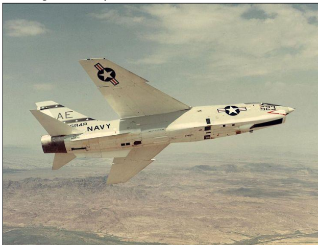
The RF-8 photo reconnaissance version that Tommy Tucker was flying the day he was shot down. Behind the black panels are the high resolution cameras.
