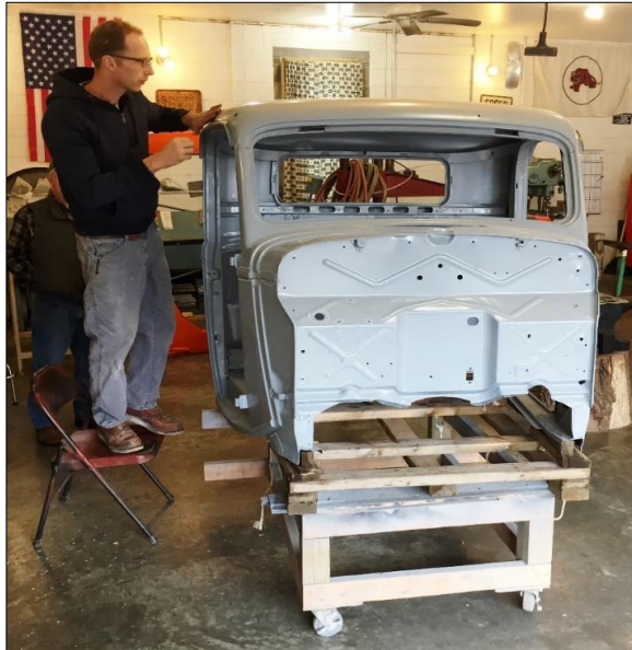
Thetan Ogle inspects and marks up the work needed to take away years of accumulated dents, patch a few holes and fix some rusty spots
