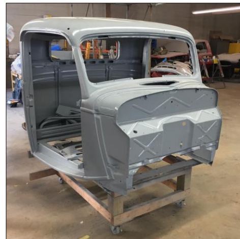
Old paint, grease and rust are gone, and the bare metal is covered in protective primer in Richie's shop
