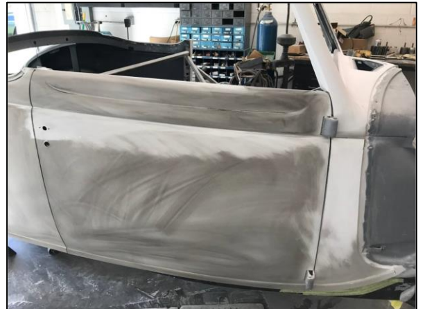
Notice the perfect door seam gap
