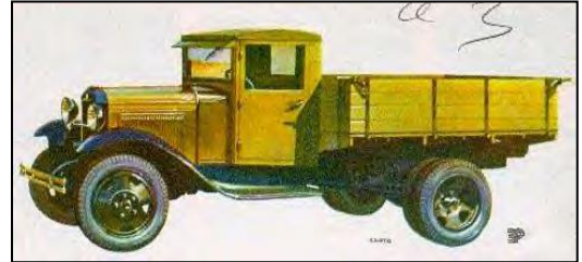
The GAZ-AA truck had a wooden cab
