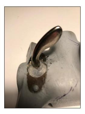
The team at AVM was then able to mask the assembly in such a way that they could put it in the nickel bath and plate only the switch. *SUCCESS* – 230 "micro inches" of electrodeless nickel. Please don't tell the judges!
