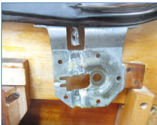
Drill out the rivets and this is what you end up with.
