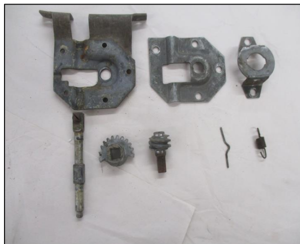
These are the parts that make up a regulator.
