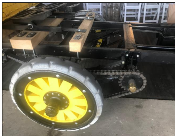
Smith Form-A-Truck installation with new axle, chain drive, and wheels
