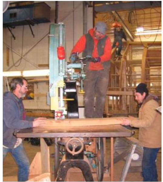
Shaping a part on the massive band saw requires three sets of hands.
