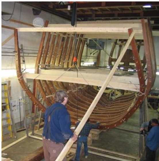
Workers install a rib – now that's a big Woodie!
