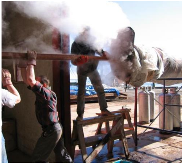
After a long time in steam, a hot board emerges from the oven.
