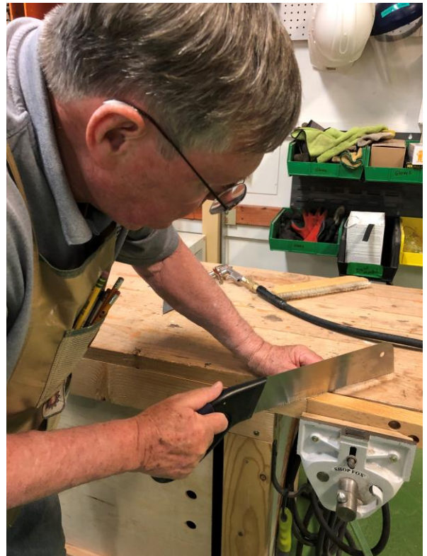
Dave using a saw with a special Japanese blade that cuts opposite most saw blades
