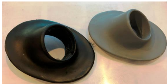
A two-piece mold for a rubber steering wheel column to firewall seal. Upper photo shows the molds, the light gray is a primer-painted original and the black rubber is the finished part. This is not available from any supplier.
