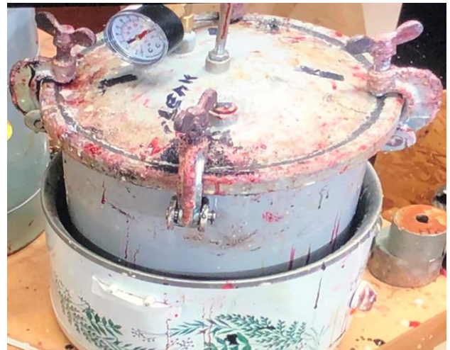
Pressure pot chamber being heated in a crockpot base used to make taillight and other lenses and similar parts.
