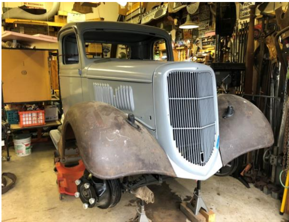
Sheet metal test fit in progress.
