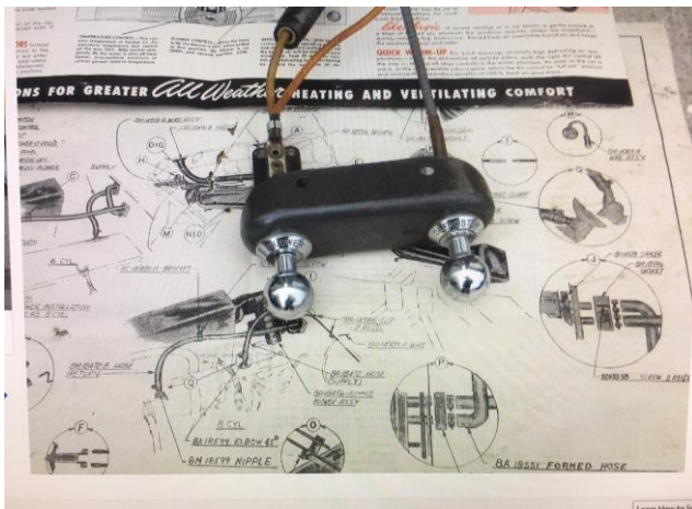
'49 recirculating heater controls
