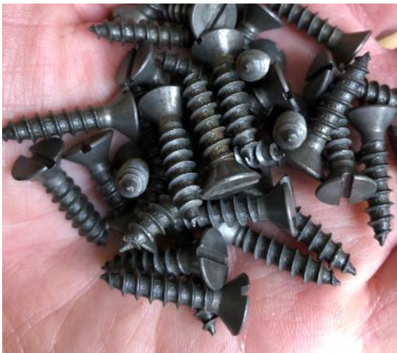
Screws with zinc plating removed
