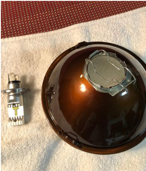
AutoPal housing made for halogen bulbs but works perfectly with LED lights
