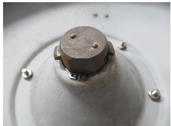
Closeup of backside of lock showing locking ears
