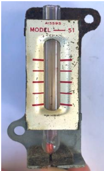
#2 – Deluxe gas gauge insert for 1935 Model 51 trucks (51-9280-B)
