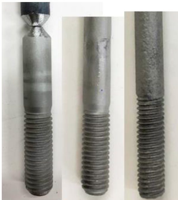
Bolt chamfered and ready for welding, finished new extension, original threaded end with longer threaded segment
