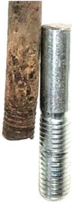
Sheared original bolt and cut-down new 1/2" bolt
