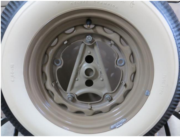
Spare carrier with cover removed – locking ears go into center hole
