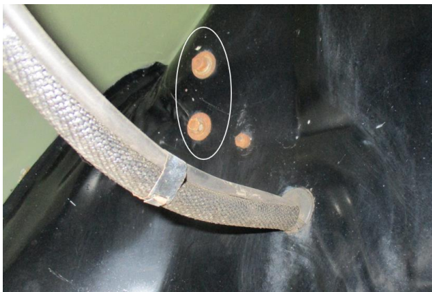
Apron support bracket bolts in early inner panel looking into the left front wheel opening
