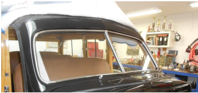
Late – stainless insert in black molding
