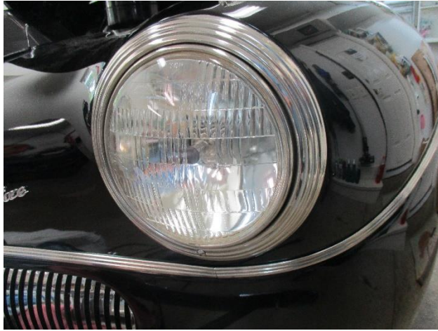
The late bezel with smooth, concentric circles
