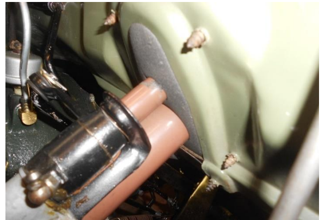
The early car has four large sheet metal screws securing the plate to the firewall from the inside; a screw lower down attaches a small tab that bridges the gap in the opening.
