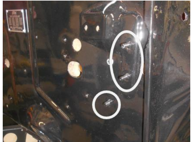
The new battery ground stud for 6-cylinder cars (circled) and the obsolete hood spring arm mounting studs (in the oblong).
