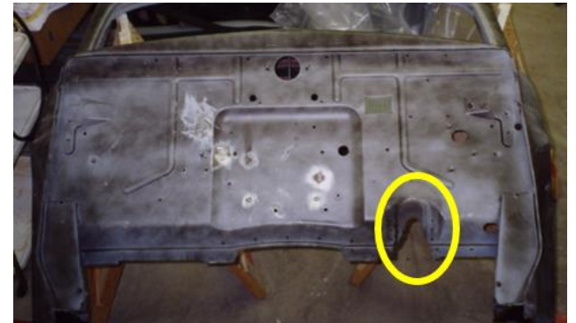
Note that the cutout in the late firewall is much smaller – still visible is the outline of the earlier, larger cutout in the firewall stamping.
