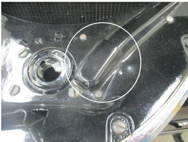
Late cover over the cable end and the spring.
