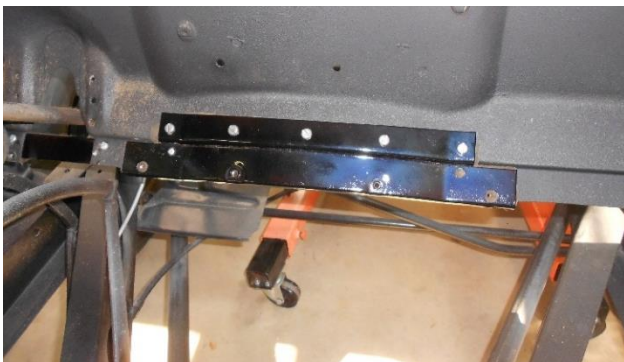
The stiffener bolted in place on the late car.
