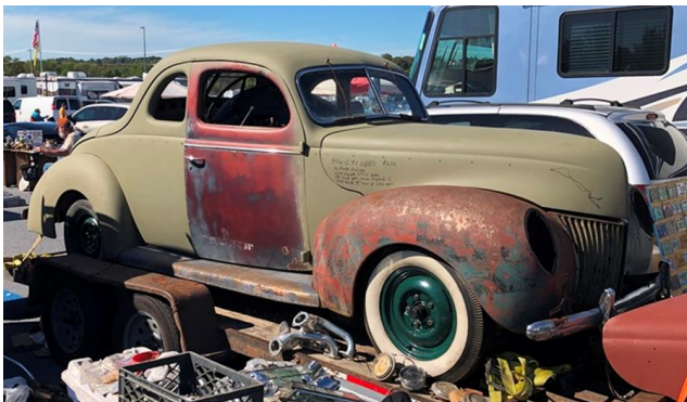
This 1939 Ford Deluxe sports a 1955 DeSoto 291-cubic-inch Hemi with a 1950 Ford open drive 3-speed and a 1959 Ford 9-inch rear end with 3.56 gears. Asking price was $20,000.
