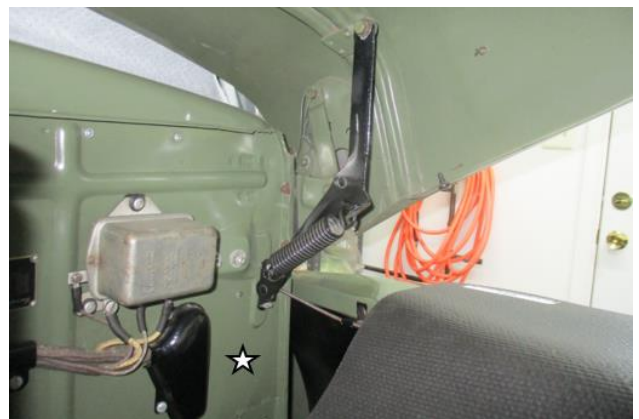
The early hood has a separate spring arm assembly mounted on the firewall. Also, remember the spot where the star is.
