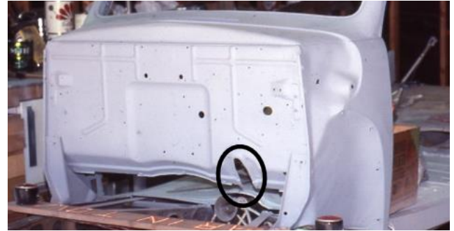
This is the cutout in the early firewall for the steering column and gearshift shaft.
