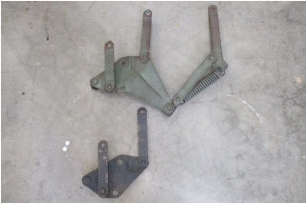
The early '41 hinge is at the bottom and the late combined hinge and spring arm assembly is at the top.
