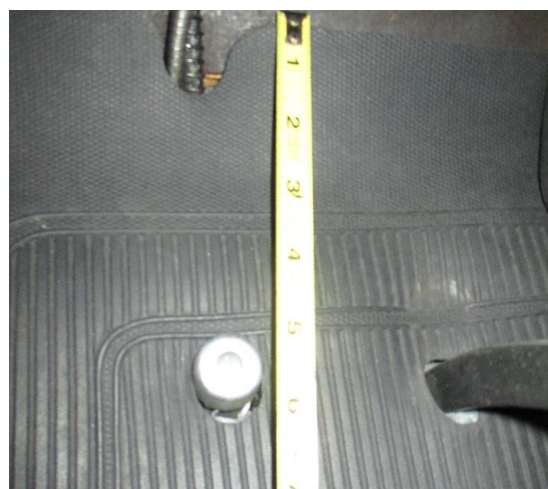
Here's the dimmer switch in the black Woodie up beside the clutch pedal arm about 5 1/2" from the front of the floor mat.
