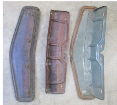
Early 2-piece vent (left) and late one-piece vent (right).
