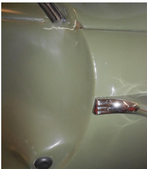
Notice that the hood rubber windlace stops at the weld.
