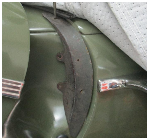
The interim strip in place on my green Woodie. With this strip installed, the windlace then extended slightly below the belt line molding.
