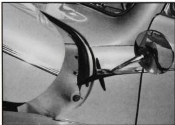
Sheet metal fillers, apparently an after thought, were added to the cowl sides to support the hood lacing.
