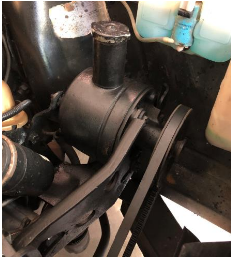
The engine compartment was nicely appointed and clean. The power steering pump looked fine on the outside, but worn bushings were allowing power steering fluid to leak out.
