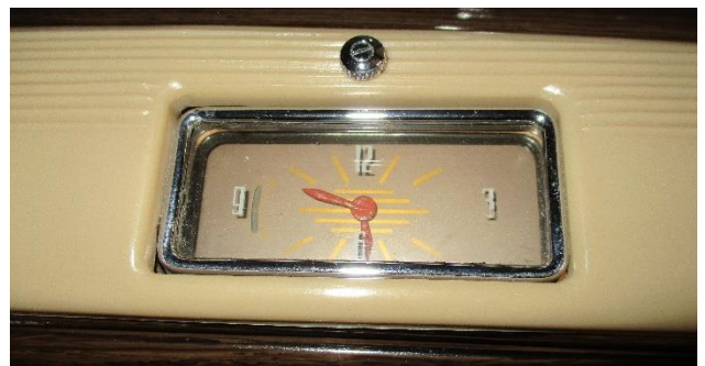
The early clock with red hands and the stem through the plastic dash trim.
