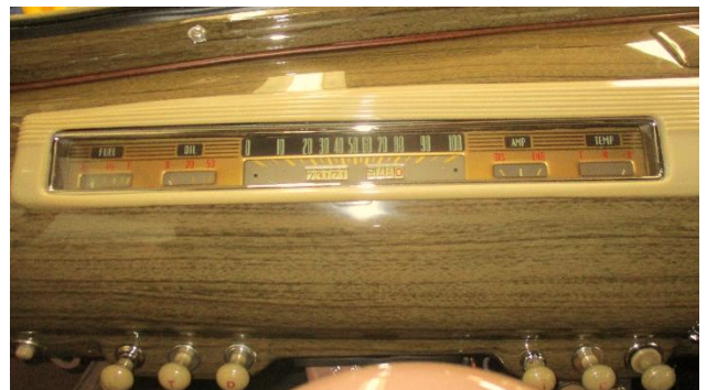
The late instrument cluster has white needles and small dash knobs below.
