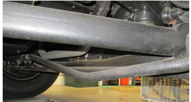
Another view of the late drag link from the right side of the late car.
