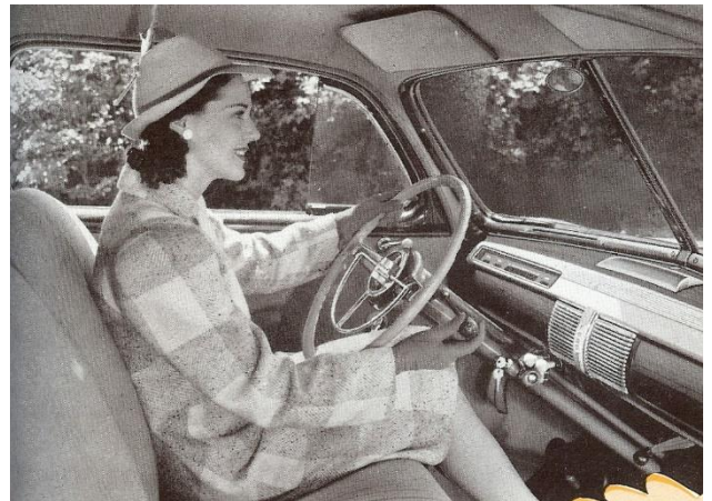
Note that the dash trim is a single piece stretching entirely across the dash. Also note that the vertical piece of chrome trim on the radio speaker grille stops when it reaches the plastic trim.
