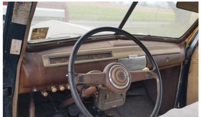
This is an early '41 dash with one piece trim. It's in a very original Deluxe Coupe that the late Bill Clatterbaugh owned.
