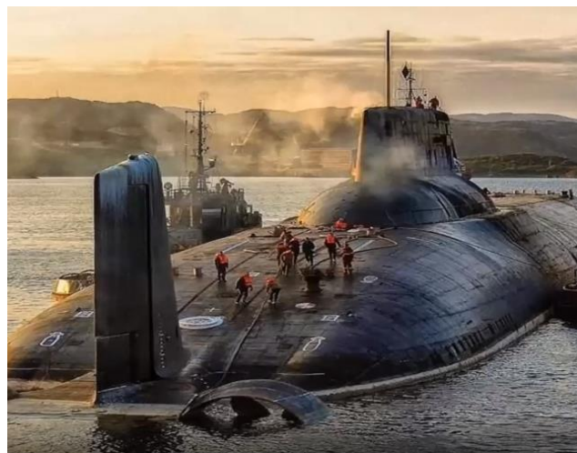
The world’s largest submarine, the Typhoon, a double submarine with missile compartments between them, is a product of the Soviet submarine design process.
