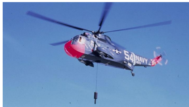
To transit more quickly between "dips" the SH-3A flew with the sonar transducer partially deployed.
