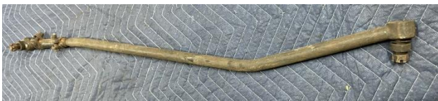
A late drag link shown as it would be when installed in a late car.
