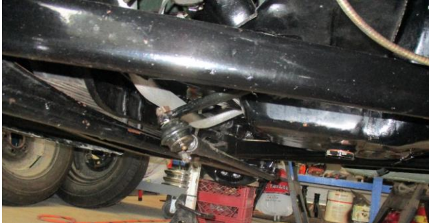
The drag link end attached to the bottom side of the steering arm on my early car.
