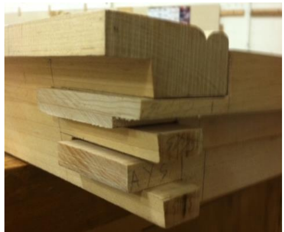
This is the type of lap joint where vertical pieces are joined to horizontal pieces like door frame or quarter panel corners.
