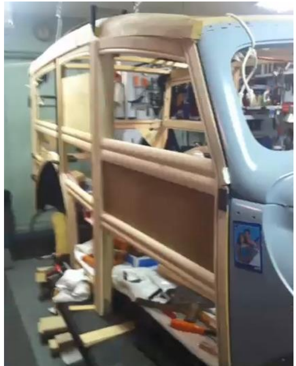
Progress on the right side with the belt line and mid-panel horizontal beams in place.
