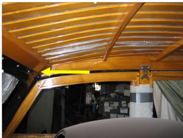
The brackets, then missing on both sides, provide extra stability where the side beams attach to the cowl assembly.
