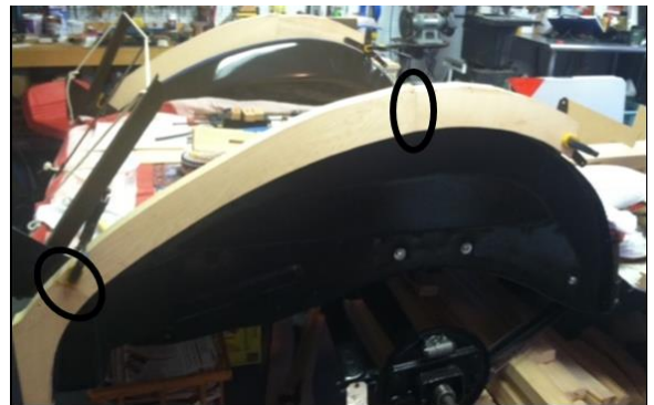
The fender arches have 3 pieces jointed together by finger joints. In this shot you can see how precisely Dave fitted the wood to the repaired fender arch.
