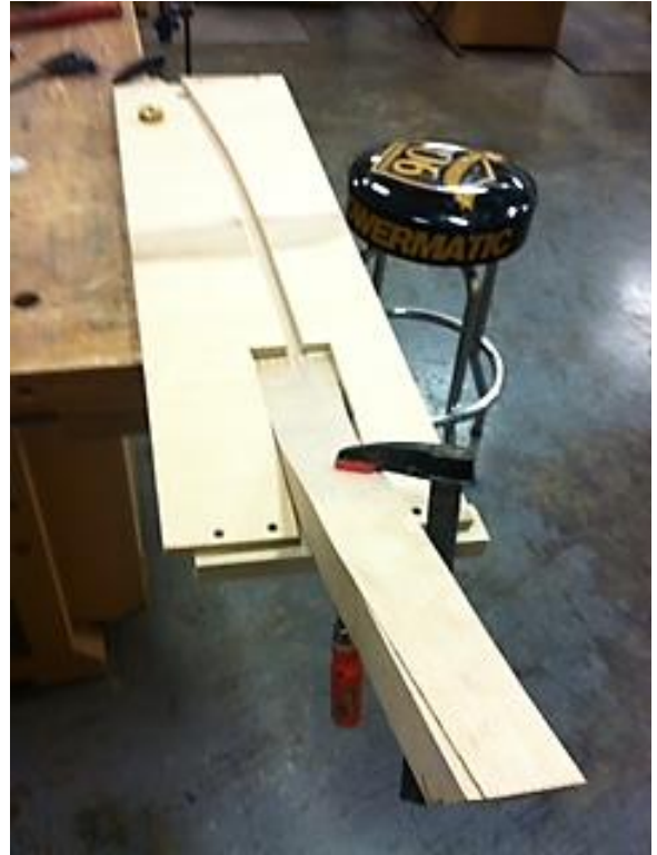
The fixture in place and ready to use a router to cut the slot.
