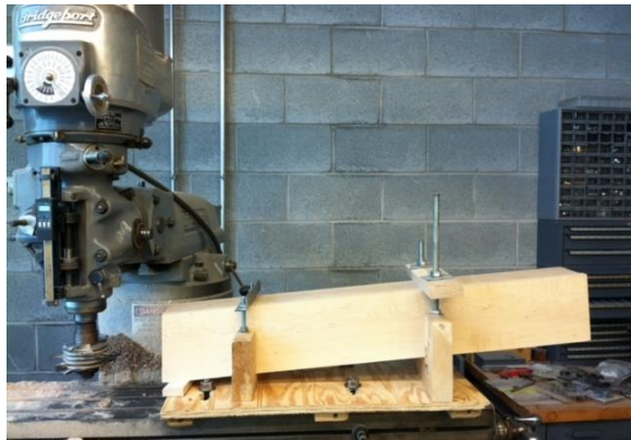
This piece needed the finger joint cut at a compound angle.
