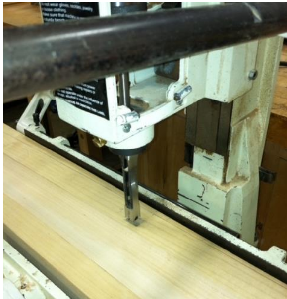
Cutting a square hole in the side beam for the roof cross bows.
