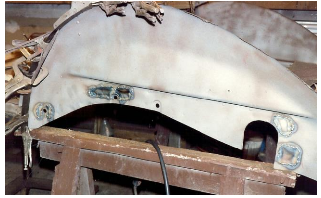
Metal moth damage to the rear inner fender wells (see below) was repaired.
