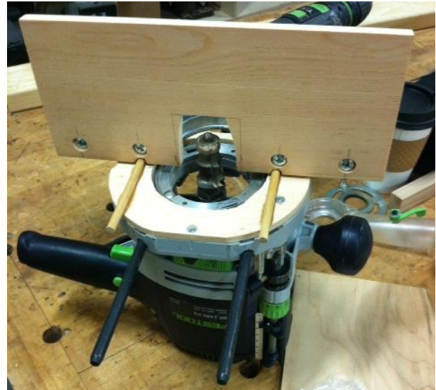
Dave designed a special fence so the router smoothly followed the fender arch profile.
