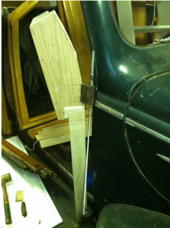
A threaded rod and a couple of nuts assured the hinges were lined up before the prototype pieces were cut for their trial fit.
