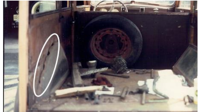
Metal moth damage to the rear inner fender wells (see below) was repaired.
