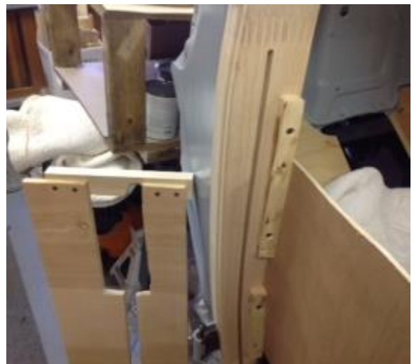
The front door post in place and the fixture standing beside it.
