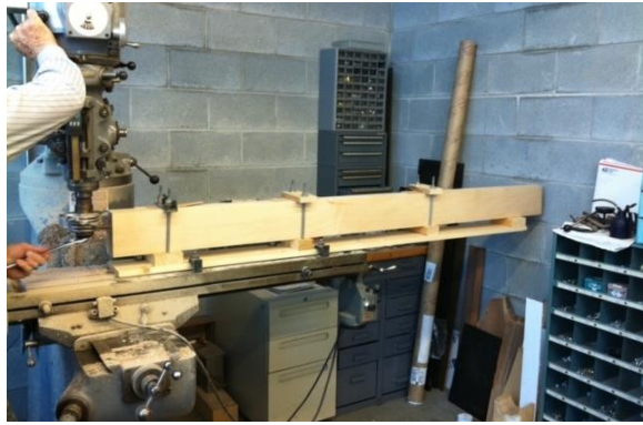
The longest single piece of the side beam (7') just fit on the Bridgeport milling machine bed when cutting the finger joint.
