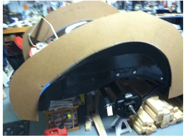
Large cardboard sheets were used to make accurate patterns for the fender arches.
