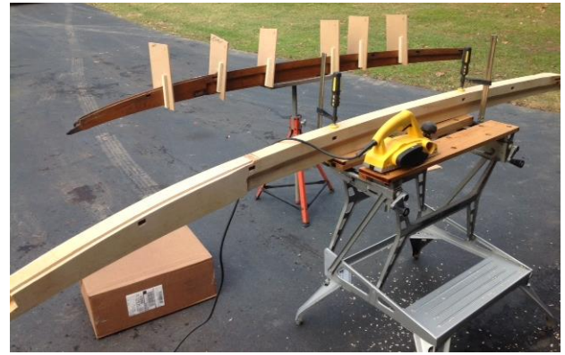
Just imaging how many different cutting operations were needed to construct a side beam. You can easily see the square holes for the roof cross beams in this picture. That's the original beam that Dave used as a pattern in the background.
