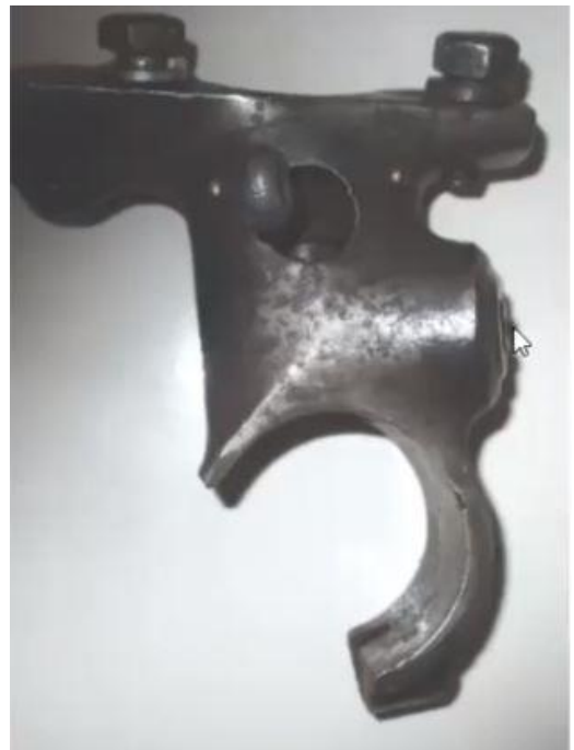
Broken column drop
