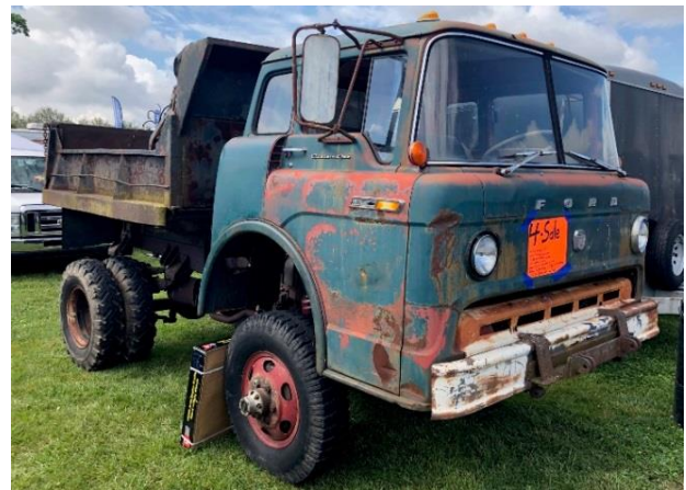
While not an EFV-8, this very cool four-wheel-drive short-wheelbase dump truck was for sale. It includes a NAPCO 4WD conversion of a 1969 Ford C-600 with new brakes, a gas V-8 engine installed, and a spare Caterpillar diesel engine and transmission are included. It "runs and drives well." Asking price is $5,500.
