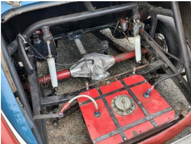
Hood up on Jimmy's car showing quick change rear
