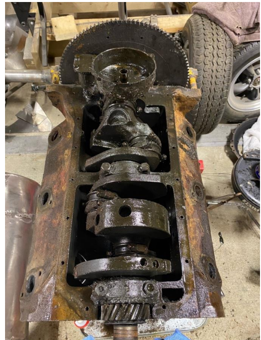
Bottom end with oil pan removed
