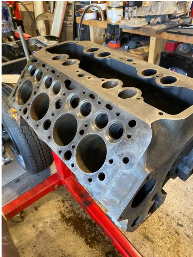
Stripped, cleaned block
