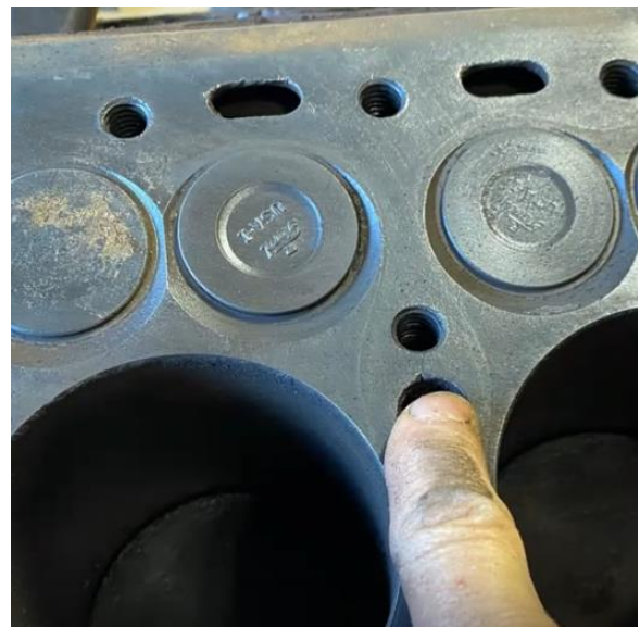
An inconsequential block crack which James plans, in the future, to have drilled and plugged
