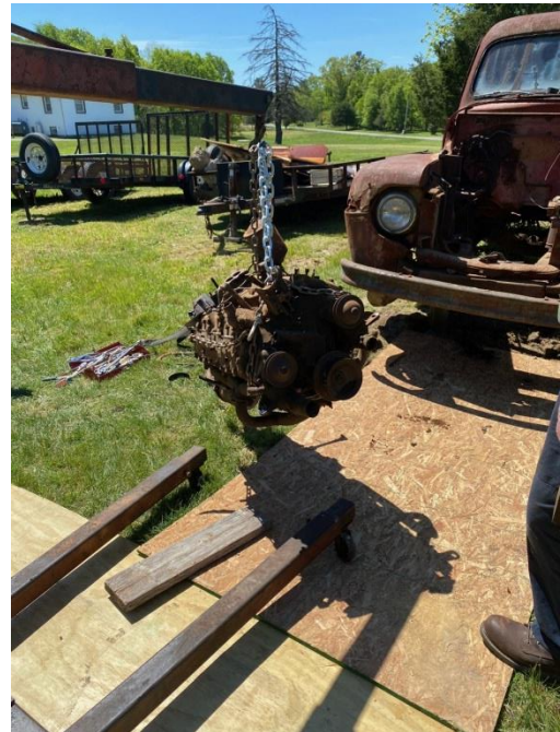
After initial cleaning, the engine comes out – cleaning continued in this position
