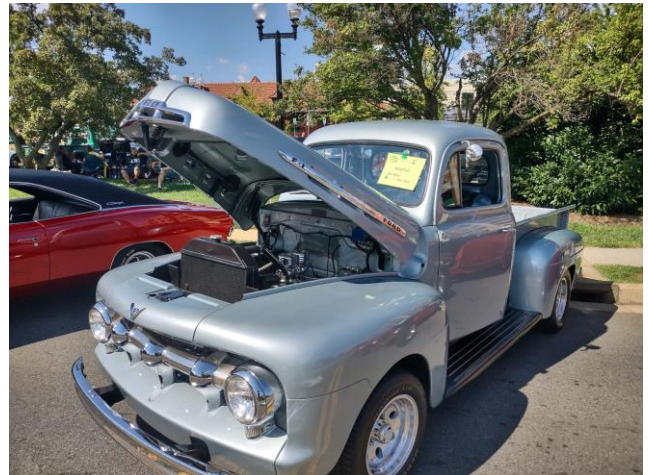
Flathead powered with F-1 with very nice aluminum heads and dual carbs
