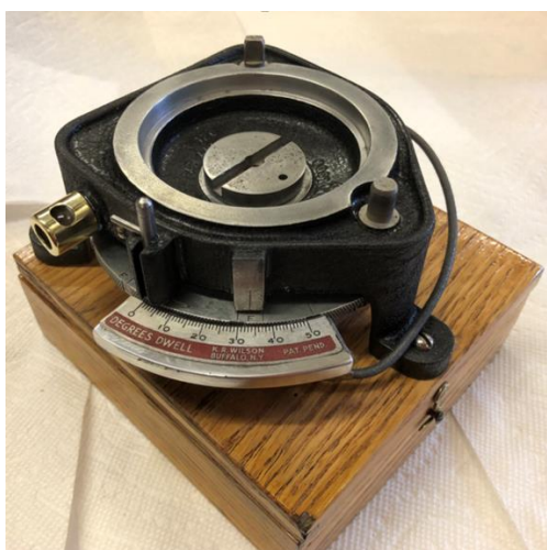
KRW distributor timing fixture (V-126) restored
