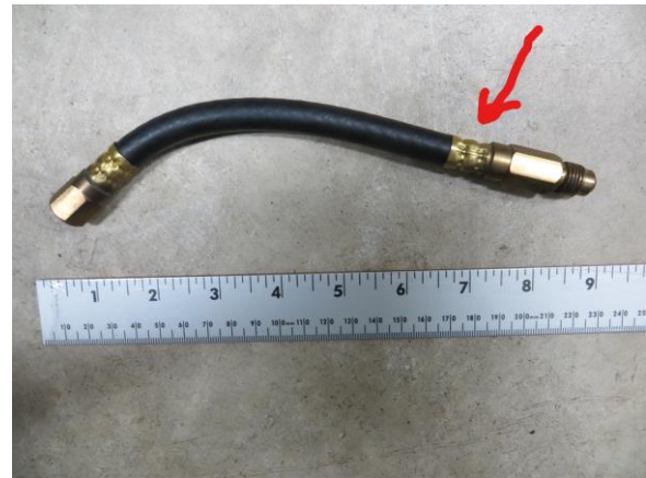
Fuel Line Failed Connection
