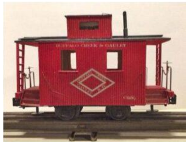
Home brew Bobber caboose with commercial wheels, journals, and couplers
