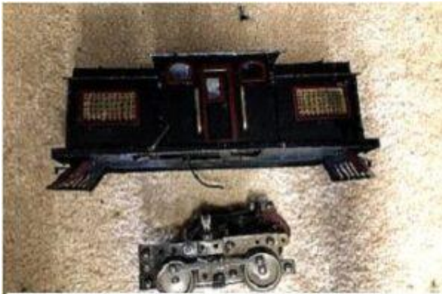
Sam, Son of STOMPER STG Yard engine History unknown. Motor modified IVES standing motor. Imbedded headlights.
