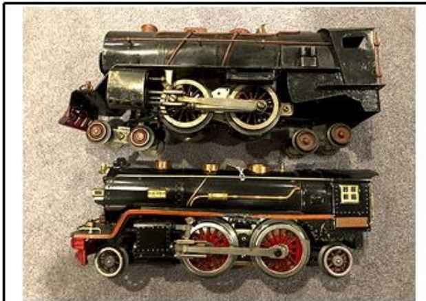
Top engine is a Lionel #390 wannabe. Motor is a Lionel #38 with modified super motor roller pickup. Hand rails and most topside trim is nonmagnetic; all painted grunge orange/brown. Lionel #384 -style tender trim is the same grunge color and is not photo-worthy. Headlight was soldered in place. Loco judged a 3.05 on backflip. Size 6.78% bigger than the shown Lionel #390. Manual disk reverse in cab. Two boiler bands.
