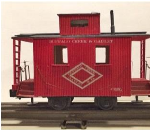
Home brew Bobber caboose with commercial wheels, journals, and couplers
