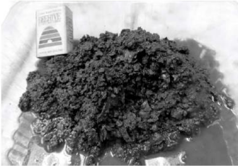
Left - Debris flushed out of my '36 block after the heads were removed. Incredibly, this was a pre-flushed and in-service engine
