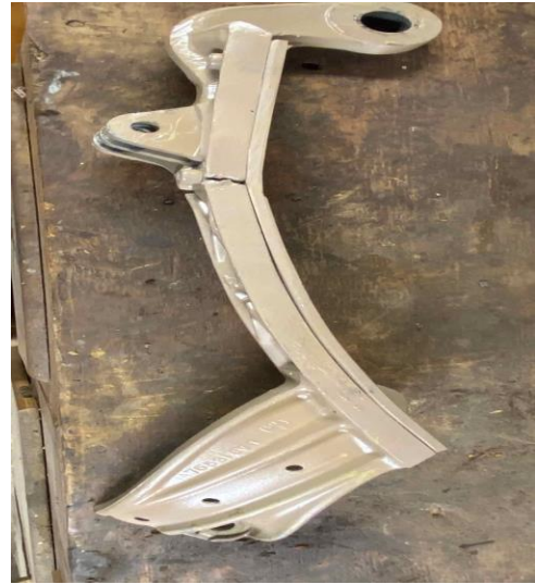
Photo of broken convertible top pieces on '51 Ford
