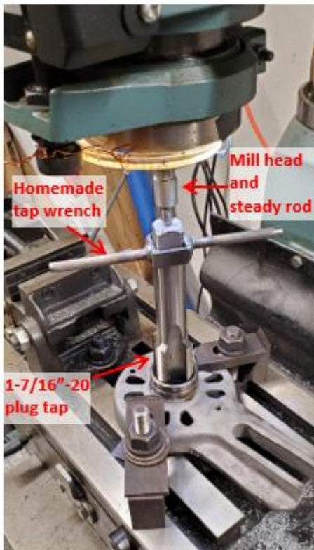
Tap held and centered with mill and end plate securely held to mill bed
