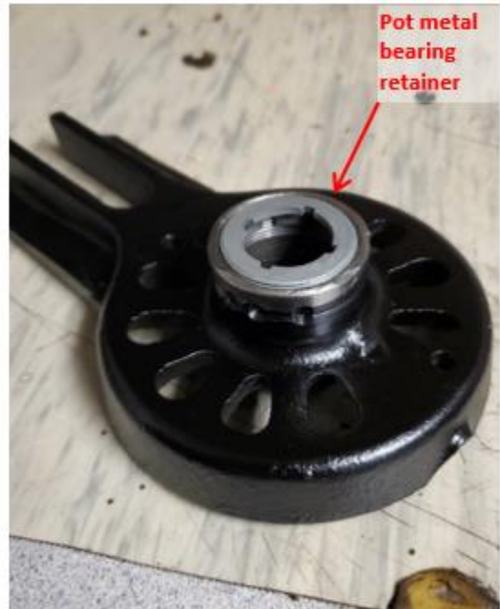
Re-threaded generator end plate with new bearing retainer partially installed
