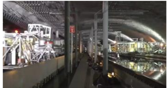
Carriages passing each other in the long test basin
