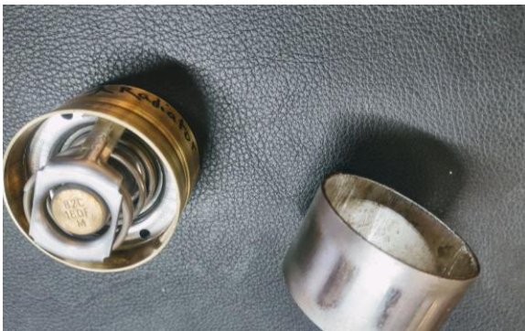
Modified thermostats with retaining sleeve concept
