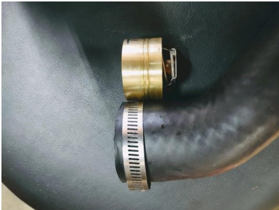
Taller thermostat didn't work in curved portion of hose
