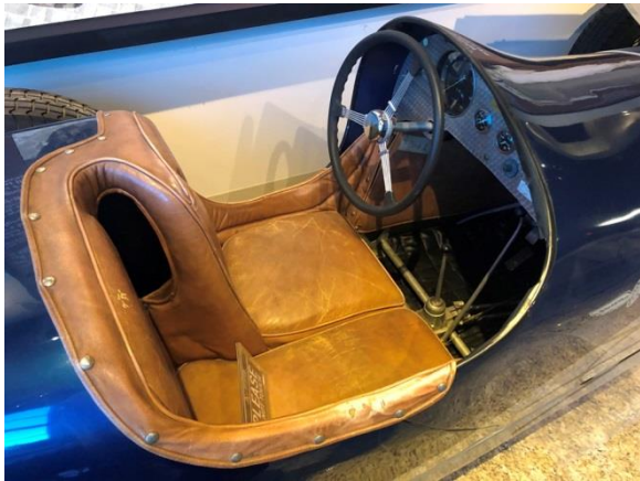
This is a 2-passenger race car. The mechanic sat slightly behind the driver and stuck his arm into a pocket behind the drive which has a grip handle.
