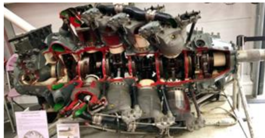
Cutaway 1930's 28 cyl. Pratt & Whitney aircraft engine
