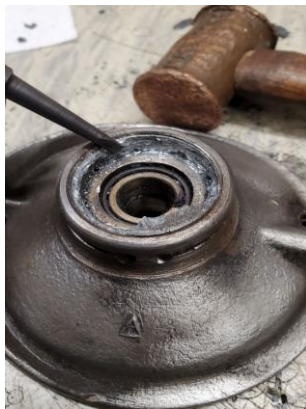
Chiseling out the bearing retainer
