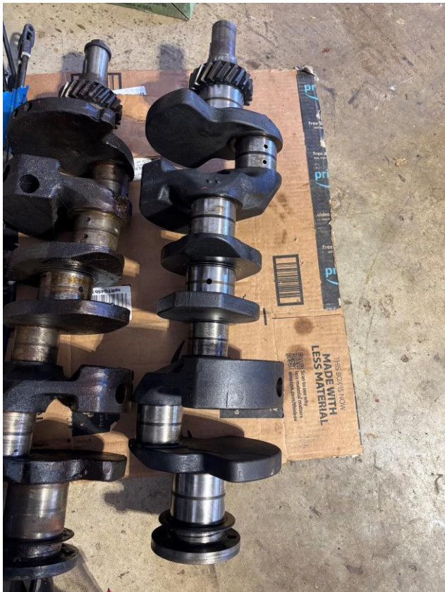
4" Mercury crankshaft on the right, sitting next to an 8BA crankshaft
