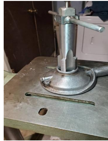
Cleaning up the bearing retainer threads
