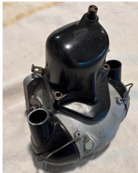
Early Ford V-8 Distributor and Coil – One of Many Tested and Calibrated by Cliff Green (photo courtesy of Chris Elenbaum)
